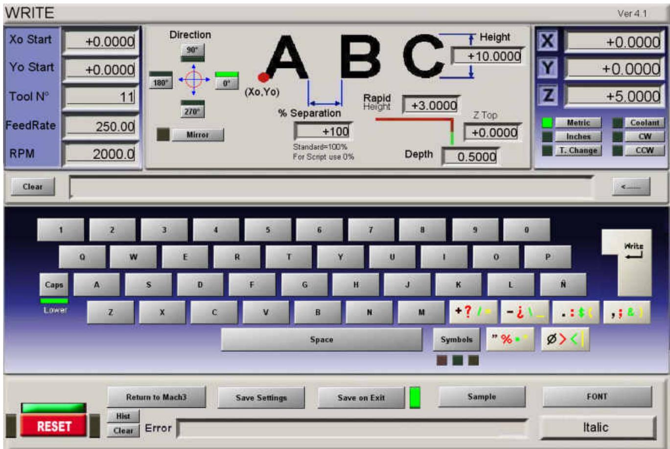
This wizard is a text engraving program for simple work like engraving part numbers and marking materials, it is not a program for doing fancy text and features.
