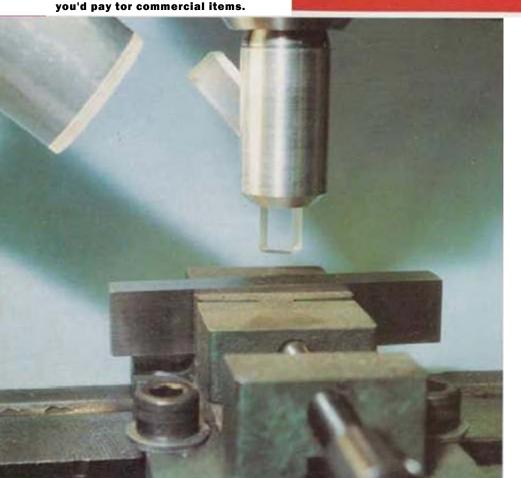
The completed optical centre-finder in the milling machine, in actual use it would be brought closer to the work than shown in otd'ar to line it up accurately
